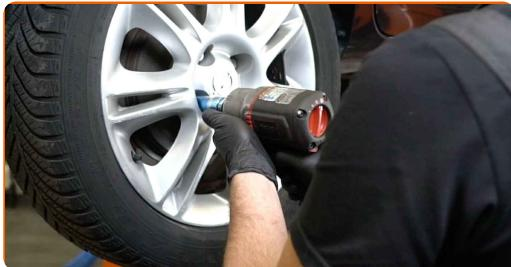
Menjava: amortizerja – VAUXHALL Corsa Mk III (D) Hatchback (S07).
