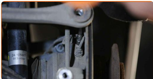
**39** Odklopite senzor ABS.
